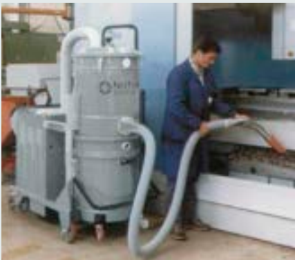
Metal sector: collection of shavings on machine tool
