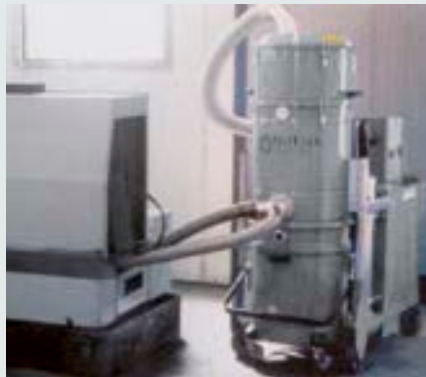
Fixed application for recovery of graphite
