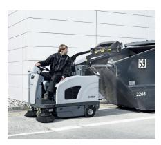
The retractable hopper can be closed from operator compartment allowing the operator to drive away immediately after dumping into a container.
