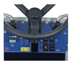
One Touch Sweeping means that brooms are only running when used. When not driving, SW4000 automatically stops all functions thus saving wear and energy
